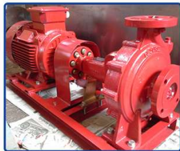
ELECTRIC FIRE PUMP
